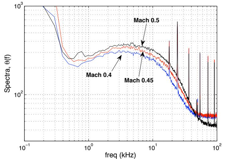
**Figure 8: Un-scaled USAFA deflection angle spectra for three Mach numbers at one elevation angle of  $116^\circ$ .**
