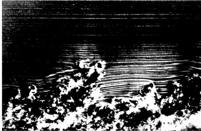
**Figure 11: Elongated vortical structures in the turbulent boundary layer, flow goes from left to right. [Ref. 18]**
