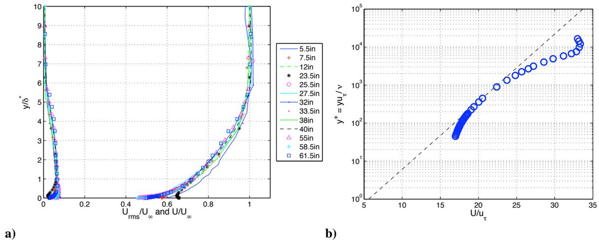
Figure 6: a) Normalized hotwire velocity profiles (mean and rms) of the upper wall boundary layer of Notre Dame transonic wind tunnel at 13 streamwise locations. b) Boundary layer profile in wall units at the optical test section. The friction velocity is 5.5 m/s. The dashed line represents the log-law, Eq. (6).
