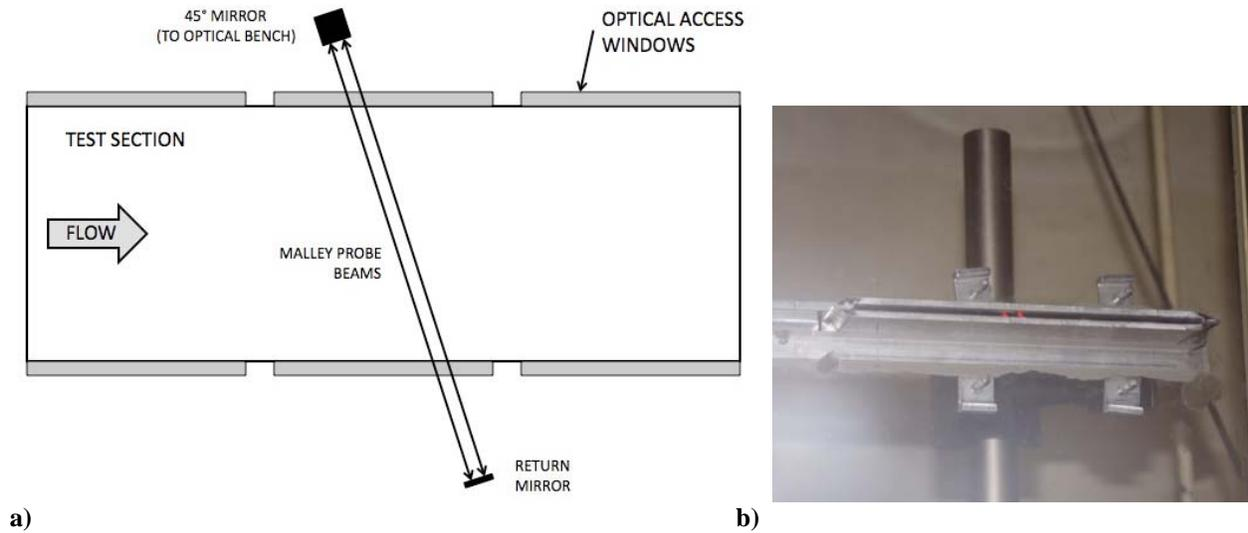
Figure 5: a) Schematic of the USAFA wind tunnel facility. b) Optical insert for USAFA tunnel.
