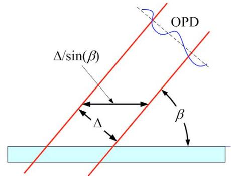
**Figure 7: Malley probe calculation of  $OPD$  for an oblique elevation angle.**
