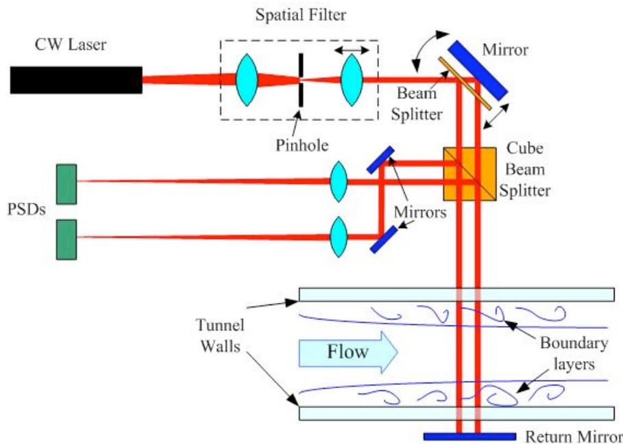
Figure 1: Schematic of the Malley probe as used with the turbulent boundary layer setup.
