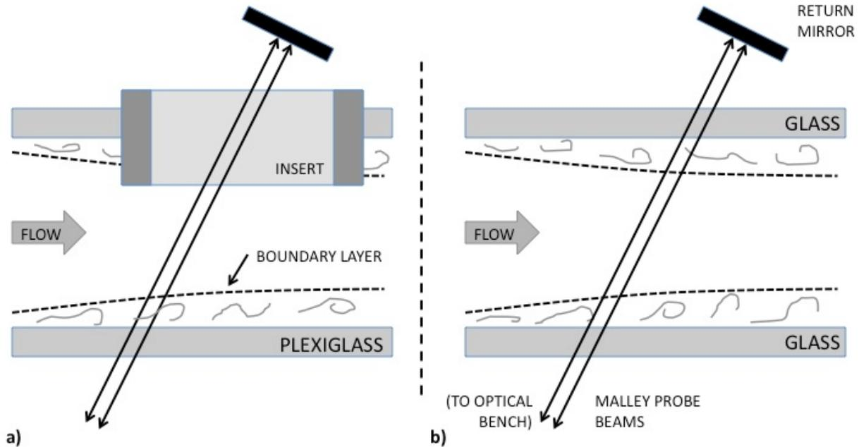
**Figure 4: Schematics of the test section for a) single boundary layer measurements with the optical insert in place to by-pass the boundary layer on one wall and b) double boundary layer measurements.**
