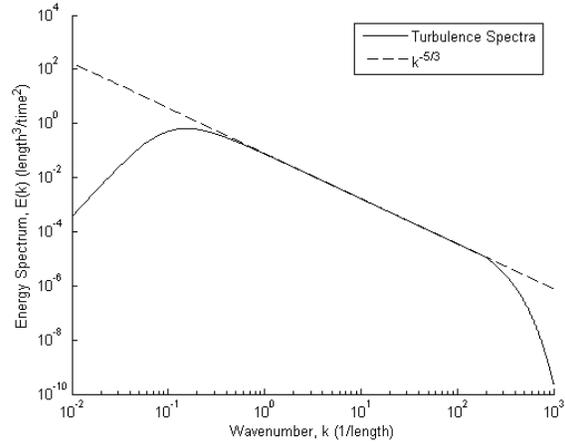
Figure 1. A sketch of a turbulent energy spectrum.
