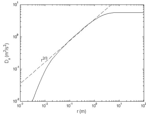
Figure 2. A structure function for velocity variations in turbulent flow.
