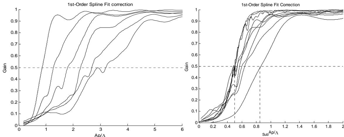
Figure 11. Results of simulated first-order spline correction (a) scaled to full aperture dimensions (b) scaled to sub-aperture dimensions.
