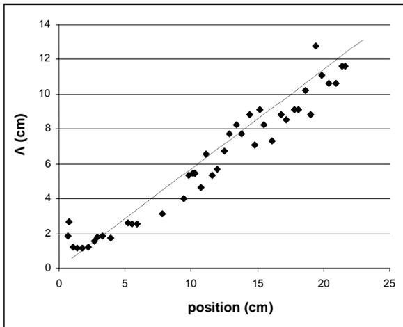
**Figure 6. Optical disturbance length with shear layer position.**
