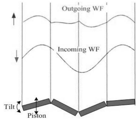
Figure 10. Segmented mirror / first-order spline correction.
