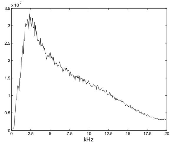
**Figure 5. Beam Jitter PSD from a compressible shear layer.**
