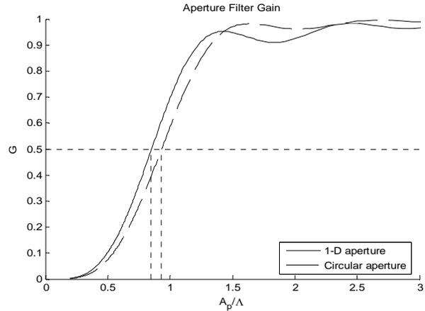
Figure 9. Effective gain for T/T correction over an aperture.
