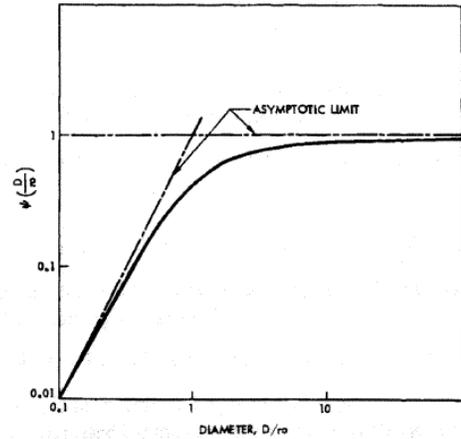
Figure 3. Fried's normalized signal-to-noise ratio.<sup>9</sup>
