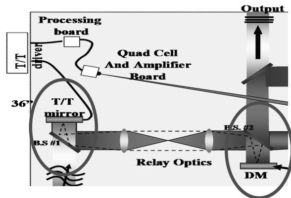
Figure 7. Two-stage optical correction in the Notre Dame AO system.
