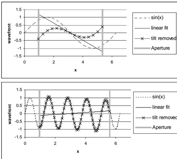
Figure 8. T/T correction for different length scales.
