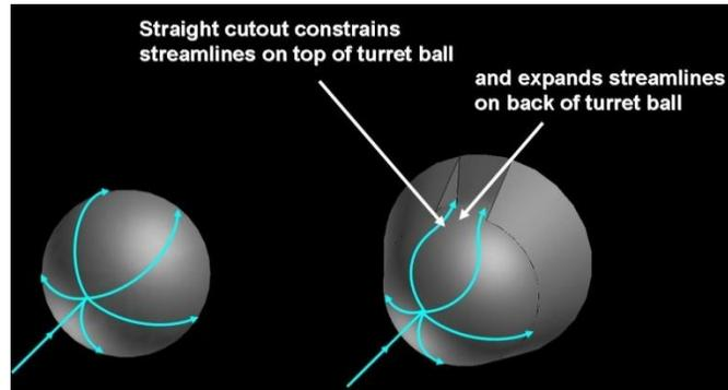
**Figure 3. Illustration showing how straight cutout walls constrain streamlines on the turret ball**
