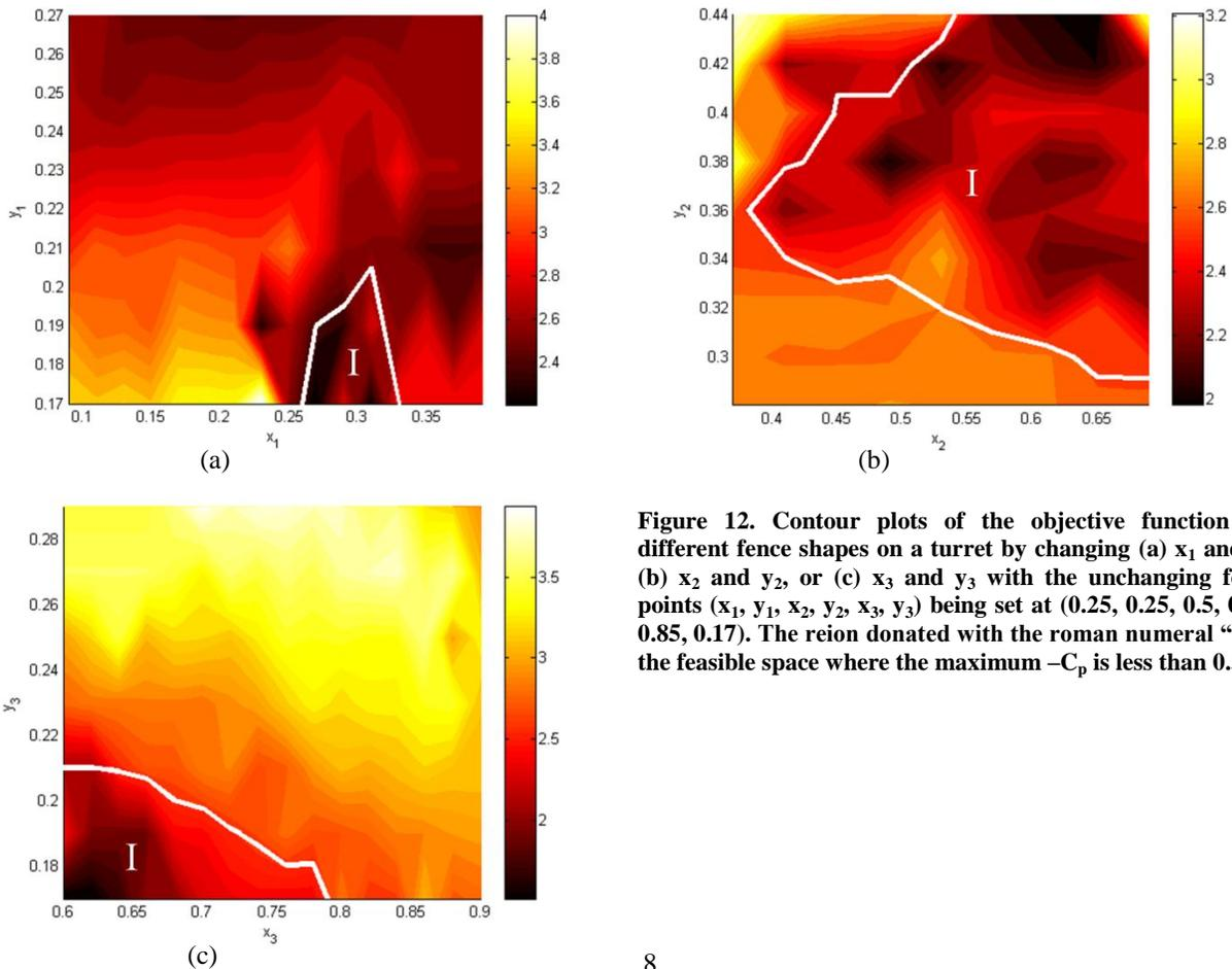
Figure 12. Contour plots of the objective function for different fence shapes on a turret by changing (a)  $x_1$  and  $y_1$ , (b)  $x_2$  and  $y_2$ , or (c)  $x_3$  and  $y_3$  with the unchanging fence points  $(x_1, y_1, x_2, y_2, x_3, y_3)$  being set at  $(0.25, 0.25, 0.5, 0.31, 0.85, 0.17)$ . The region denoted with the roman numeral “I” is the feasible space where the maximum  $-C_p$  is less than 0.5.
