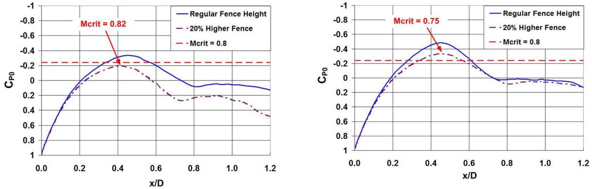
Figure 8. CFD-computed pressure distributions around turret ball for 2 different fence heights at a lookback angle of 40 degrees (left) and 60 degrees (right).
