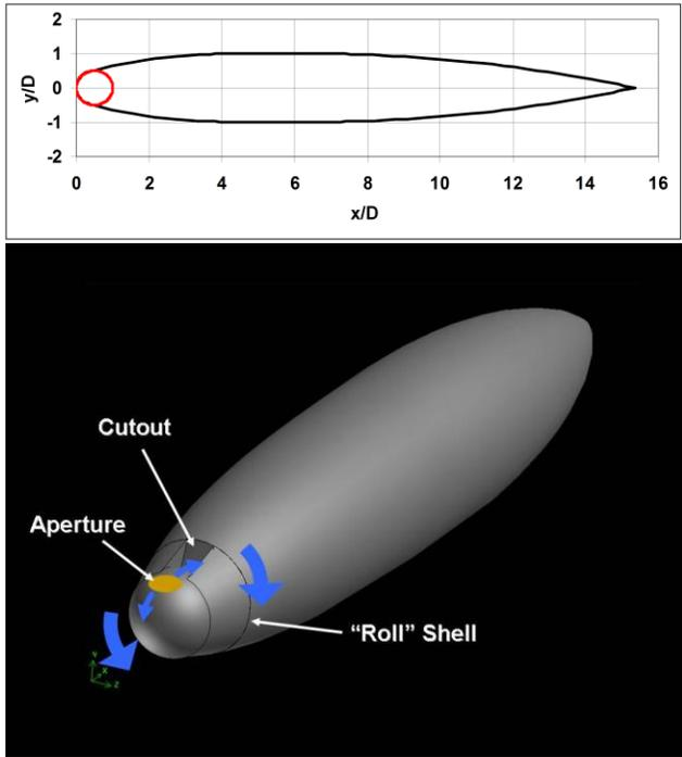
**Figure 2. Cubic forebody fairing shape in 2-D (above) and 3-D (below). The turret ball is shown as the red circle at the nose of the front of the pod.**
