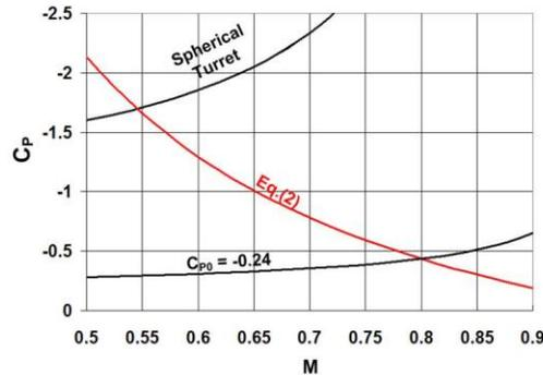
Figure 1. Critical Mach number for spherical turret, and minimum  $C_p$  for cruise at  $M = 0.8$ .
