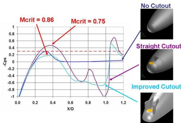
Figure 6. CFD-computed pressure distributions around turret ball and critical Mach numbers for different cutout configurations at 20 degree lookback.
