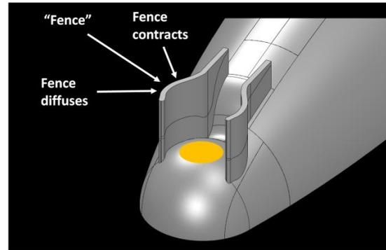
Figure 5. Top part of pod with improved cutout and fence to control flow around aperture.
