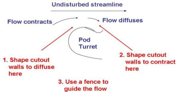
Figure 4. Diagram showing how cutout wall shaping can improve the flow, and aero-optic environment around the turret ball.
