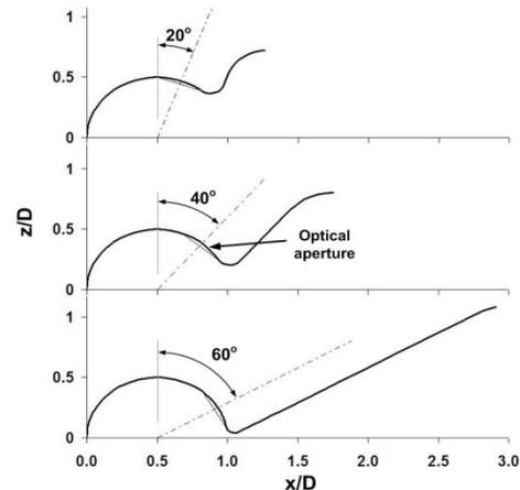
Figure 7. Centerline geometry for different lookback angles.
